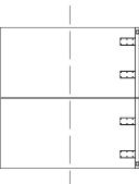
3. Attach hat channels 1/3rd of the way from the front of the worksurface.
