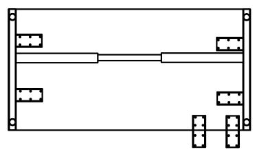
4. Attach Open frame leg to end of the return
