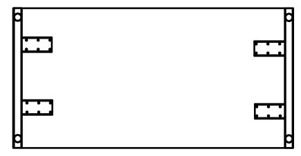
2. Attach work surface support bar 1/3rd of the way from the front of the worksurface. Expand outside portion of each side of the hat channel to fit in the gap between surface and leg. Tighten down center bolts.
