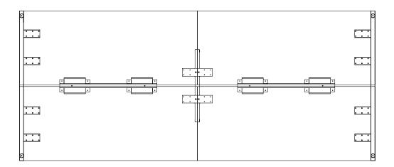
9. Attach mending plates on the outside of the shared legs, approximately 2 inches from the outside edge of the worksurface
