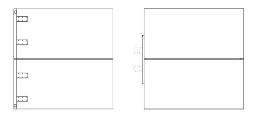
7. Attach screen clamps to the trough. Discard small pin that comes with clamp. Make sure they are secured tightly and parallel to the edge of the trough.
