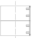
3. Attach hat channels 1/3rd of the way from the front of the worksurface.
