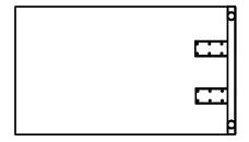
5. Flip return rightside up and rest free end of return against and under mending plates. Align with outside corner and attached top to open side of mending plates.
