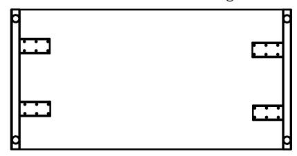
2A. Attach work surface support bar 1/3rd of the way from the front of the worksurface. Expand outside portion of each side of the hat channel to fit in the gap between surface and leg. Tighten down center bolts.
